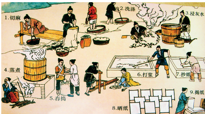
Figure 1.4.5: A picture showing how paper was made in the Han Dynasty.
